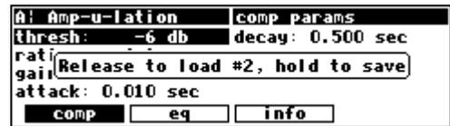
If you release the button immediately, the operation will be canceled, and the previous setup saved under that button (if any) will be loaded.
