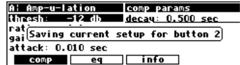
When a setup is saved under an encoder button, the names of its presets will be displayed when the button is first pressed. If the button is immediately released, the setup will not be loaded.
