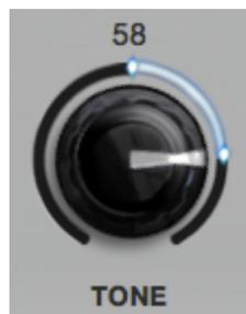
Some rotary knobs can not be mapped to the expression pedal. If one of the values of a knob would cause the algorithm to be controlled directly by an expression pedal for example, that rotary knob is not allowed to be mapped to the expression pedal. If a rotary knob cannot be mapped to the expression pedal, the light ring around it appears as greyed out.
