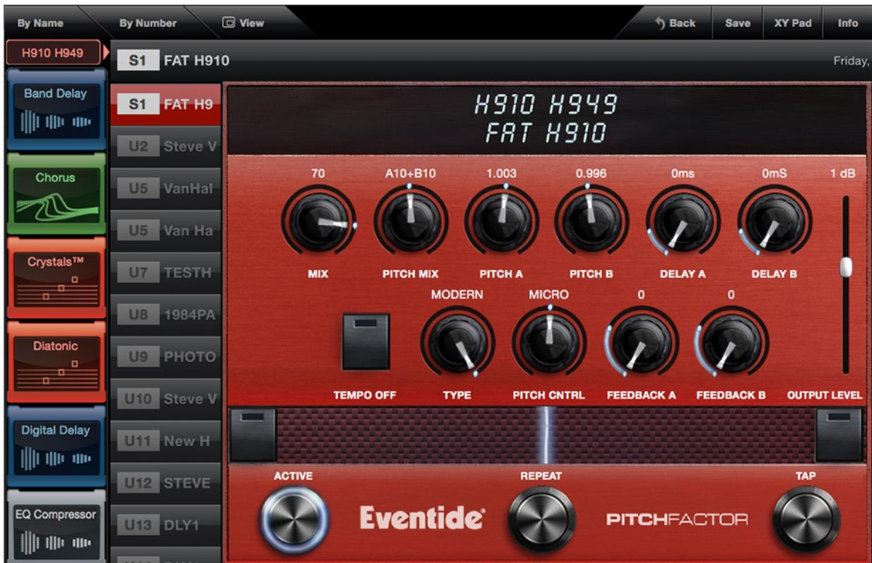
You can select a different preset in this screen to assign to the active preset position by simply pressing the button for another preset, and you can save your preset assignment by clicking the save button in the toolbar above the preset control interface.
