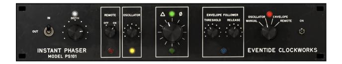
**IN/Out** Bypasses the plug-in. Out for bypass, In for wet output.
