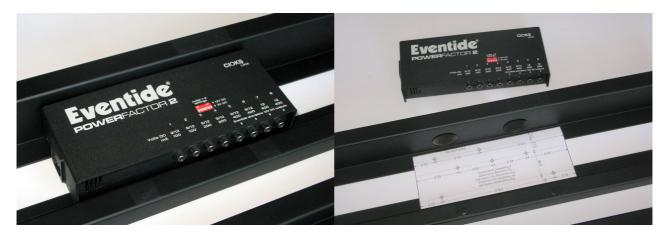
Secure the template to the board using some Scotch tape. Use a centre punch to mark the positions of the four holes to be drilled.
