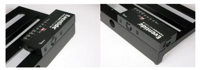
Prior to top mounting you should remove the detachable rubber feet from the power supply. Use the template to mark the three holes indicated with yellow on the template for mounting the power supply flush with the back of the pedal board. Drill the holes and fasten the unit using just the screws. For top mounting you don't need the spring washers nor the stand-offs.
