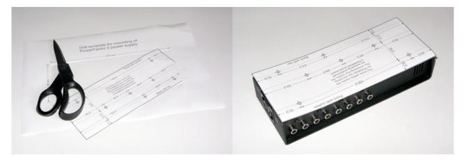
Now you have to decide where to mount the power supply in terms left/right. One of the two recommended positions is close to the middle of the board where the fan is facing one of the holes in the back of the board as shown below.
