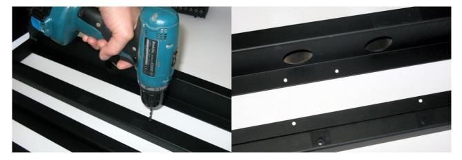
Now use the four screws to attach the power supply to the board. Use the included hex key to tighten the screws. Now you're done and ready to make all the connections with Flex cables. On the following pictures you see the PowerFactor 2 mounted underneath the Pedaltrain pedal board from different angles.
