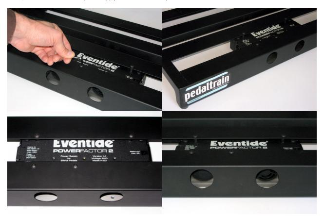
If you wish to mount the PowerFactor 2 power supply underneath a bigger Pedaltrain board like PT-3, PT-Pro or PT-Grande models, the procedure is the same. In case of these bigger boards you're more free to choose where to place the power supply in terms left/right, since there's free space on whole length of the board for letting the ait from the fan pass through.
