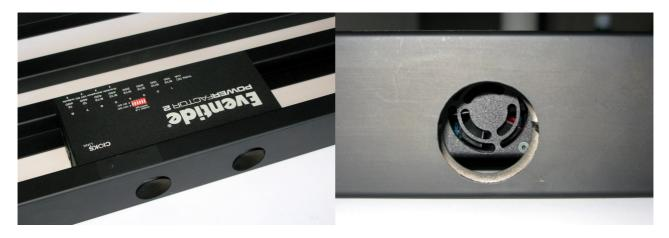
On the left picture below you see the position close to the middle of the board. If you wish to extend the PowerFactor 2 with additional power supply from CIOKS link range, you should place the PowerFactor 2 further to the left. Now the fan is facing the second hole in the back of the board. In this way there's enough space to link the PowerFactor 2 with ex. CIOKS Schizophrenic power supply using the link adapter.
