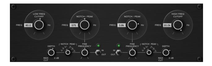
**Low Freq Cutoff** Sets the 3 dB cutoff point of the low pass filter. The filter sup-
