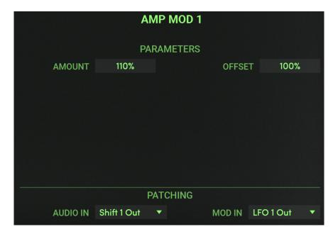
The Amp Mod blocks are similar to synthesizer VCAs Use these blocks to smoothly modulate audio signal levels creating auto-panning, ducking and other dynamic effects.
