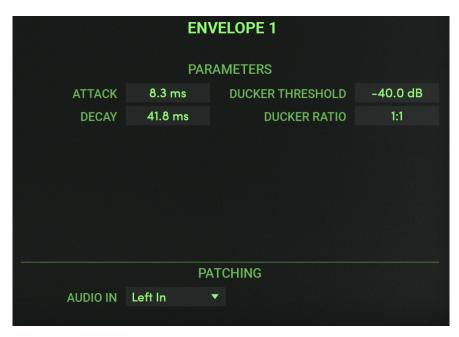
Two independent envelope generators are available to create output in response to changes in the input signal. Two outputs are generated: an envelope follower output (the left output jack) and a ducker output (the right output jack). You can use these outputs to have any parameter (such as pitch shift) be controlled by the loudness of a signal.
