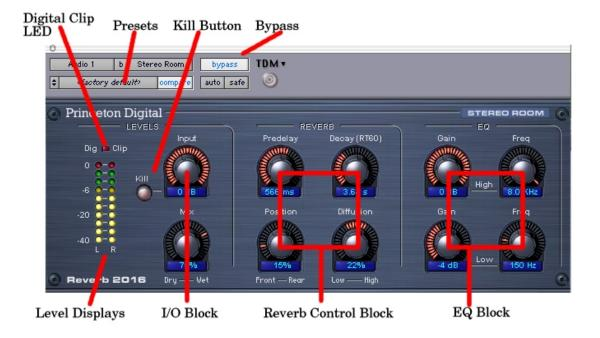
The image above is of the Stereo Room plug-in for the Stereo-In to Stereo-Out mode. In the Mono-to-Mono mode there's only one level display. The Plate and Room plug-ins also have only one level display, but otherwise appear and function identically to Stereo Room.
