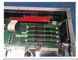
Remove 2 screws and lock washers from motherboard
