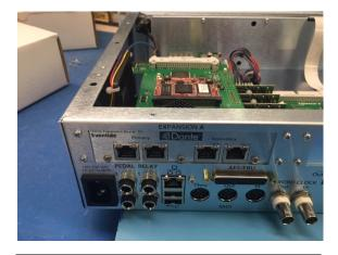
Attach 4 screws into expansion slot "A". Install top cover back onto unit
