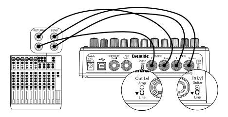
When connecting ModFactor to a Mixer, set ModFactor's Input and Output Level Switches to "Line."
